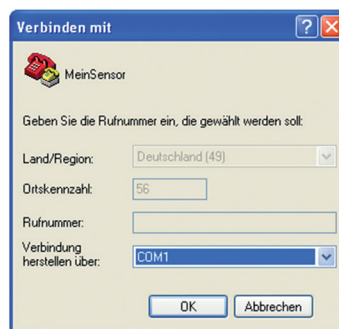
Fig. 10: Microsoft Windows Hyper Terminal Choice of the interface for communication. Here COM port. 1.
